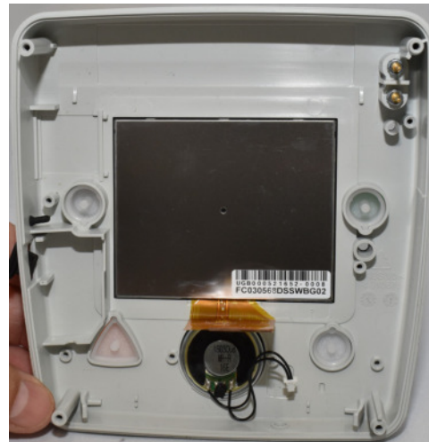
Housing with LCD complete 4.600143 see 9.3 Setup new LCD with older device, page 63
